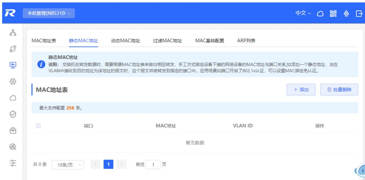
The screenshot shows the "静态MAC地址" (Static MAC Address) tab selected in the navigation bar. A tooltip provides information about static MAC addresses. Below it is a table titled "MAC地址表" (MAC Address Table) with columns: 端口 (Port), MAC地址 (MAC Address), VLAN ID, and 操作 (Operation). The table displays the message "暂无数据" (No data available). At the bottom, there are pagination controls showing "共 0 条" (0 items total), "10条/页" (10 items per page), and a current page indicator "1".
