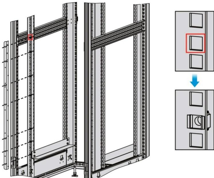
**图2-7 机柜式挂耳安装示意图三**
